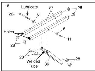
19. Lubricate an M10 x 115mm Bolt (55). Slide an M10 Washer (6) onto the Bolt.
